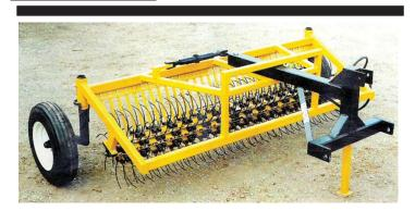
The KIRCHNER SWATH FLUFFER lifts & fluffs a swath of hay, grain, or other crops, so that air gets under the swath to dry or cure it faster. This cuts the number of days or hours between cutting, baling and harvesting.
